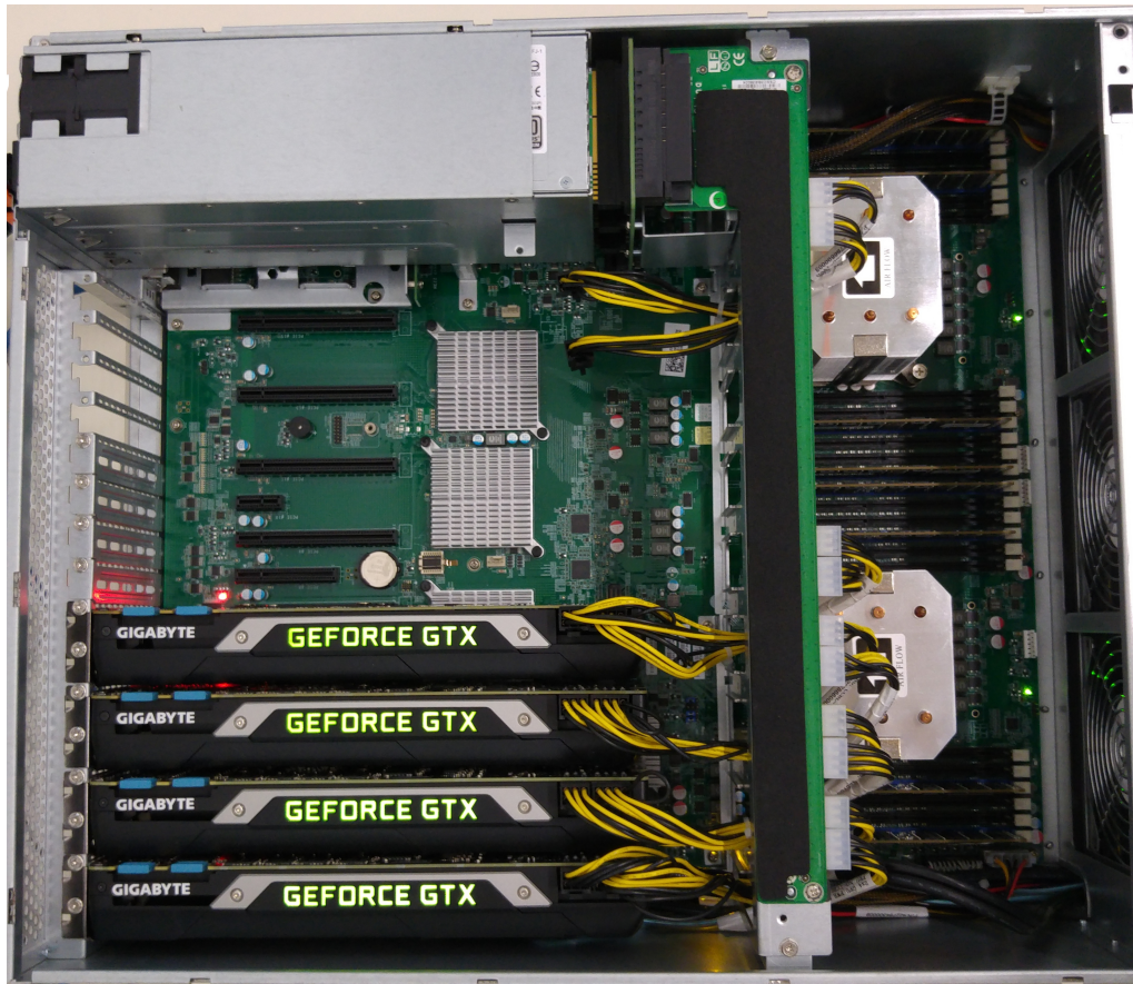
Figure 6.1: A view on the test system as used to evaluate the Multi-GPU implementation, featuring four GeForce Titan X GPUs driven by two Xeon(R) CPUs. (Source: RCPE GmbH)
