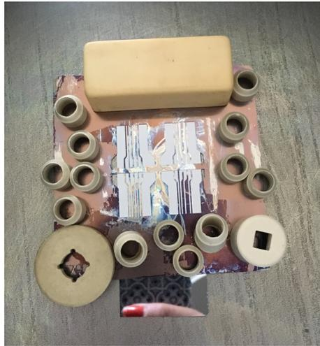
Figure 13: Direct lithography in the reactor. Mask is weighted with ceramics during the deposition.
