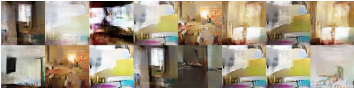
Figure 3.4: Samples from a Generative Adversarial Network exhibiting mode collapse trained on LSUN [76] bedrooms. Multiple similar images are generated in the same minibatch instead of a diverse set of samples. Image taken from [3].
