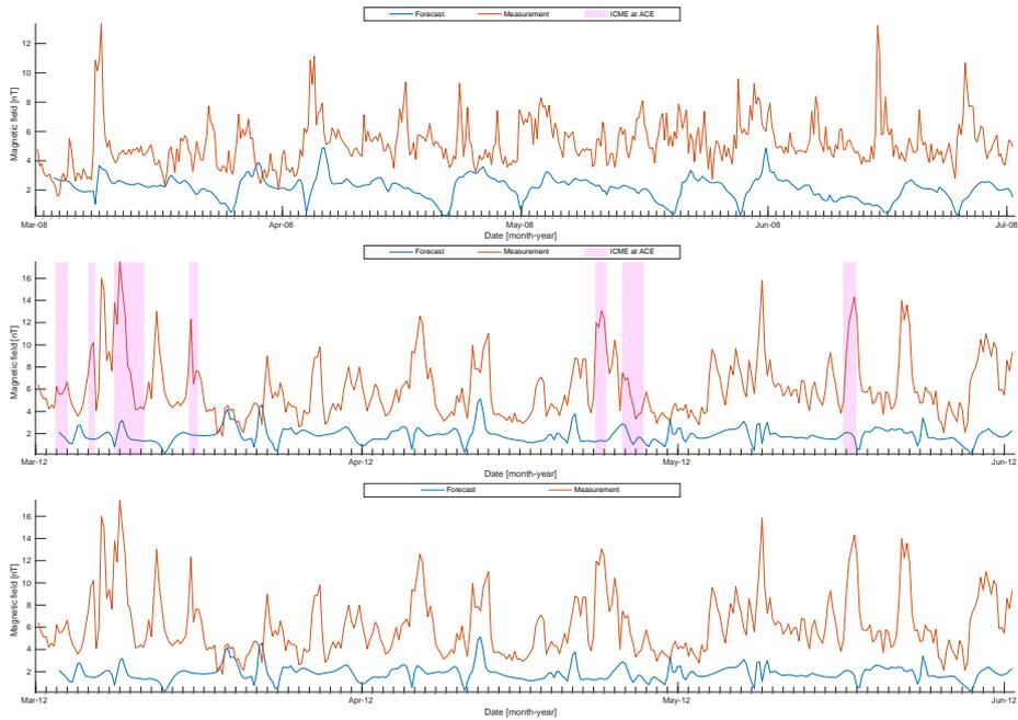
**Figure A.31.:** Solar wind total magnetic field obtained by ACE (orange curve) for 2008 (top), 2012 (CME rejected, middle), and 2012 (CME not rejected, bottom) in comparison to the EUHFORIA total magnetic field forecast where the central region is shifted to +2 days.
