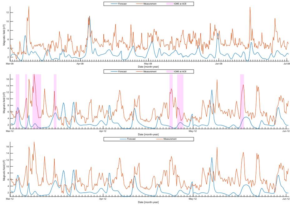
**Figure A.38.:** Solar wind total magnetic field obtained by ACE (orange curve) for 2008 (top), 2012 (CME rejected, middle), and 2012 (CME not rejected, bottom) in comparison to the ENLIL solar wind total magnetic field forecast.
