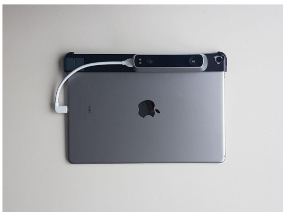
Figure 6.1: Ipad with attached Structure sensor.
