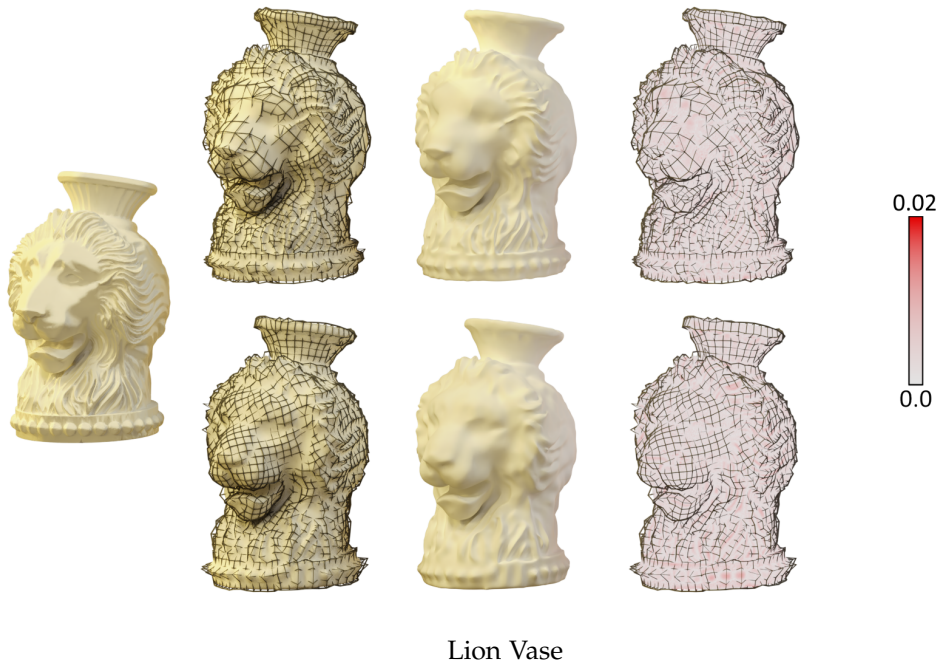
Figure 5.3.: A comparison of the results of Jakob et al., 2015 and the work of this thesis. The extracted quad-dominant meshes have about the same number of vertices and are both transformed to subdivision control meshes with the method in this thesis. On the left are the surfaces resulting from scan captures. 2nd from left: The subdivision control meshes generated from the scan data. The limit surfaces derived from control meshes are shown (3rd from left) before colouring the error between the scan data and limit surfaces (right). The top rows show the results of the method presented in this thesis. Their control meshes are dense in regions where it is required to capture fine detail, but coarse in low-curvature regions. The resulting limit surface shows a lot more detail when compared to the bottom rows, which shows results from Jakob et al., 2015's method, which is more isotropic. As a result, the bottom limit surfaces contain considerably less detail and the errors to the scan data are larger.
