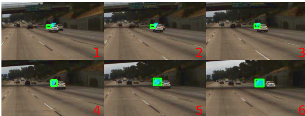
Figure 5.8: Sample of a tracking failure (621 from the training data). Mask (blue) and MRCNN bounding boxes (green) are shown.
