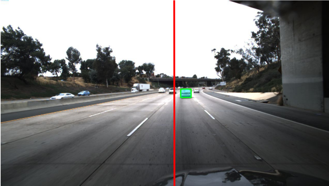
Figure 4.4: x=c_x (red line) and a vehicle at d_Y = 0.05 m (green bounding box). The vehicle coordinate center is not in line with the principal point, since the camera is not mounted centrally on the vehicle or panned accordingly.
