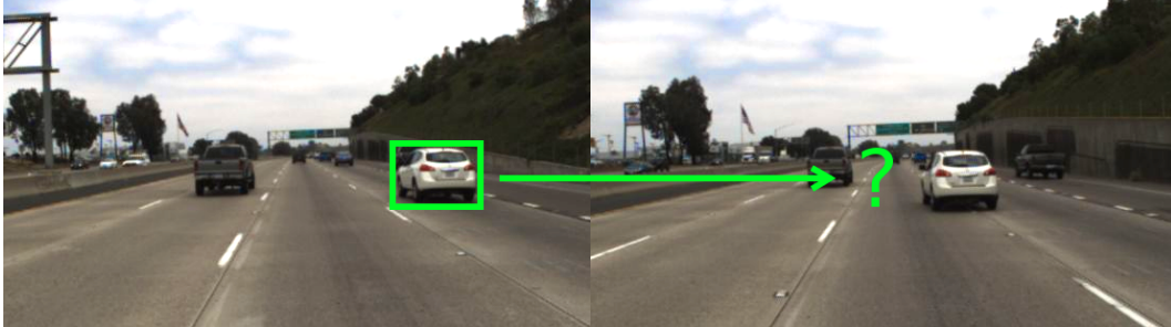
Figure 3.1: Basic concept of object tracking. The highlighted car on the left has to be found in the picture on the right.
