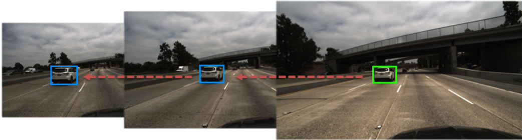
Figure 4.6: Tracking the vehicle in the rightmost frame (green bounding box, known) backwards through time (blue bounding boxes are calculated).
