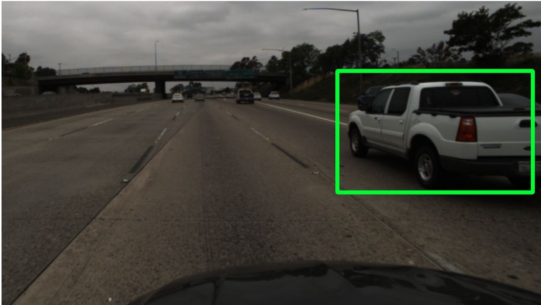
Figure 4.7: Example of an imprecisely annotated bounding box. The ground truth bounding box does not tightly enclose the vehicle.
