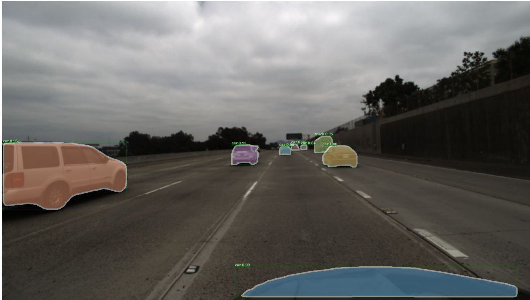
Figure 4.8: Sample output of MRCNN segmentation masks, class labels and confidences.
