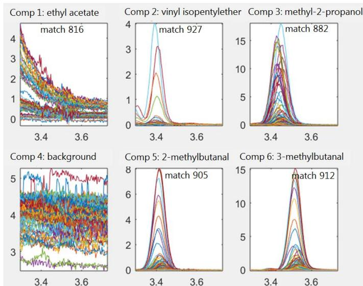
**Figure 4:** Weighted elution profiles (not overlaid) from a 6 component PARAFAC2 model applied to the data shown in Figure 3. Identifications and match factors from search in the NIST database are also shown.
