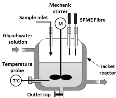
**Figure 1:** Schematic diagram of the saliva reactor
