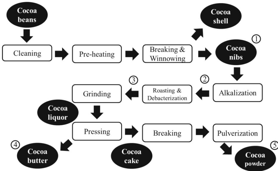
**Figure 1:** Cocoa powder process (numbers indicate sampling points)
