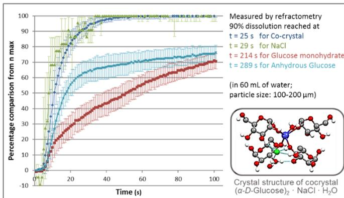
**Figure 3:** Dissolution kinetics of co-crystalline glucose sodium chloride vs. its individual pure ingredients indicating that the co-crystal dissolves faster than glucose or glucose monohydrate alone.
