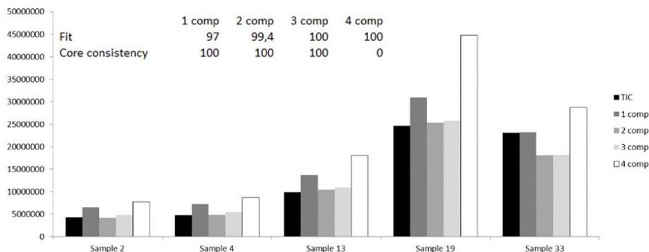
**Figure 5:** Peak areas of 2-butanone in five selected samples. The peak areas were calculated from TIC's using standard integration settings in ChemStation and by applying 1, 2, 3 and 4 component PARAFAC2 models.
