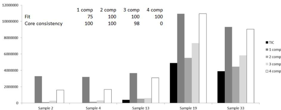
**Figure 6:** Peak areas of 3-methyl-2-butanone in five selected samples. The peak areas were calculated from TIC's using standard integration settings in ChemStation and by applying 1, 2, 3 and 4 component PARAFAC2 models.
