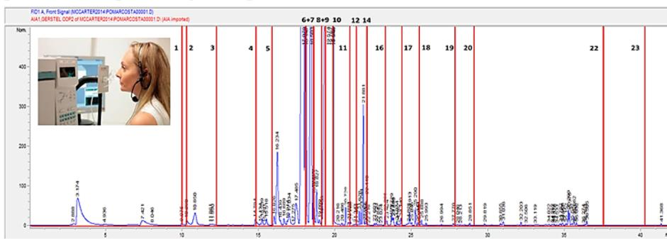
**Figure 1:** Gas chromatogram + olfactogram of orange juice volatiles (production without inert gas (O<sub>2</sub>), 0. month of storage) obtained by HS-SPME coupled to GC-FID/O. The numbering verticals, marking olfactory responses corresponds to Tab. 1.
