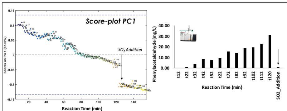
**Figure 3:** PCA results for the NIR data obtained during the reaction time. A) Scores of PC1 versus process time plot. B) Phenylacetaldehyde concentration measured by GC-MS during reaction time (each 10 minutes)
