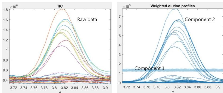
**Figure 1:** Total Ion Chromatograms (TIC) from the interval 3.71 - 3.99 min from 40 chromatograms and weighted elution profiles from a PARAFAC2 model with two components
