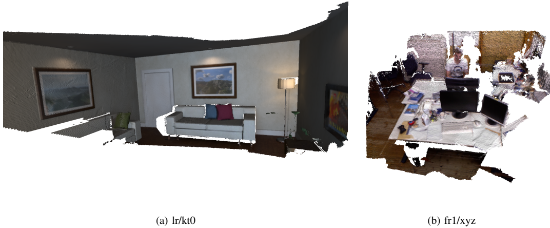
Fig. 5: Sample reconstruction models of our approach from the TUM RGBD and ICL-NUIM datasets.
