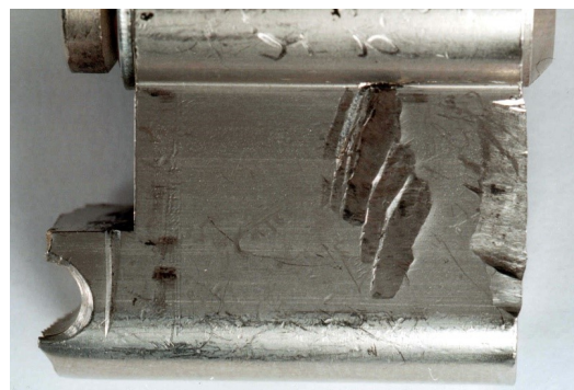
Fig. 1: Snapped lock with multiple toolmarks.
