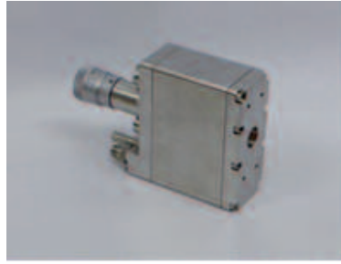
Figure 1. Piezoelectric-driven supersonic pulsed valve with displacement enlargement mechanism.
