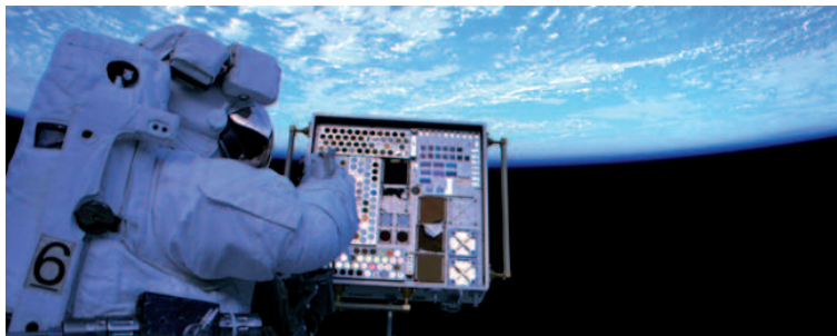
Figure 1. MISSE-1 PEC-1 Pallet attached to the ISS after 1 year of exposure (Photo by NASA).
