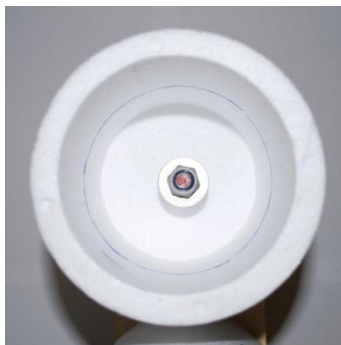
(a) Formwork with threaded rod in the lower half.
