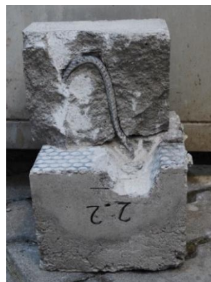
(b) Exposed reinforcement in the upper half of the specimen for a better visibility of the deformations.
