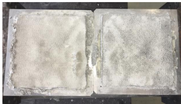
Figure 6.31: Representative fracture pattern of the series S3.
