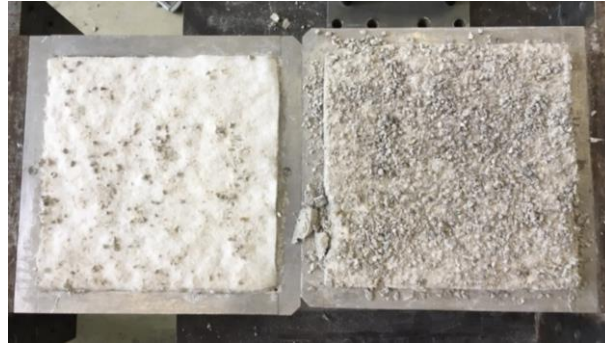
Figure 6.32: Representative fracture pattern with additional fine gravel on the fleece.
