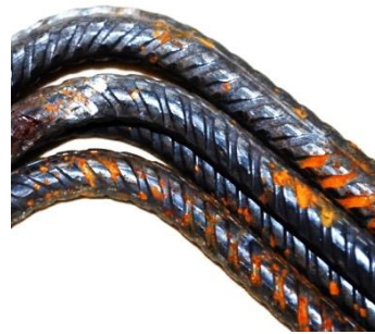
(b) Reinforcing steel BSt 550 Ø10.
