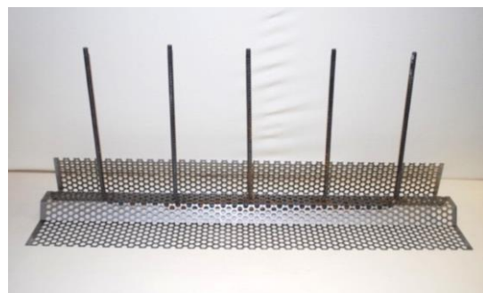
(d) Connecting element with completely installed connection reinforcement.
