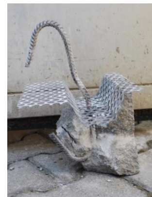
(c) Exposed reinforcement in both halves of the specimen for a better visibility of the deformations.
