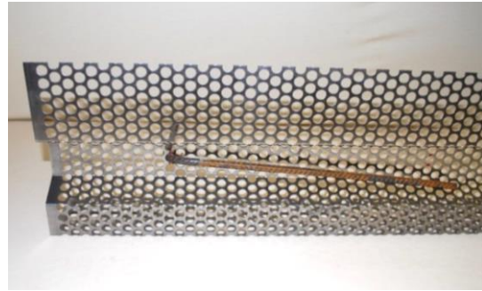
(b) Connection reinforcement is inserted through the holes of the perforated metal plate.
