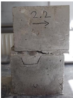
(a) Representative fracture pattern after the shearing process.
