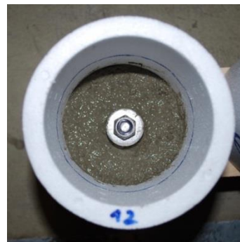
(b) Layered filling of the formwork and subsequent compaction.
