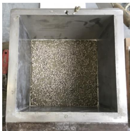
Figure 6.16: Surface of the shear joint of series S4.
