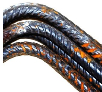
(b) Reinforcing steel BSt 550 Ø10.
