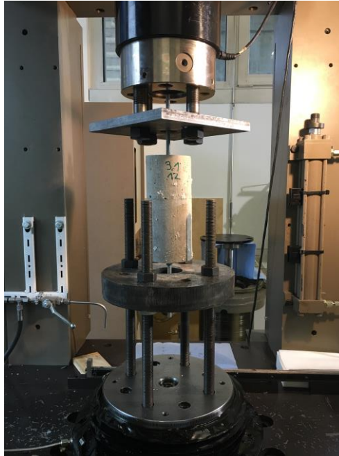
Figure 6.3: Test configuration of tension test.
