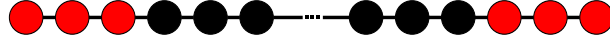
Figure 10: Graphical representation of a system in chain geometry (black sites) coupled to two baths in chain geometry (red sites). The bath sites couple with each other but only one bath site couples to the system.
