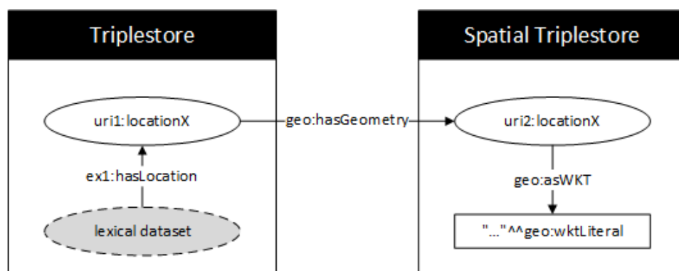
Figure 3.2: A graph representing a location with its spatial information stored on a separate source.
