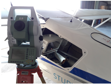
(a) Total station
