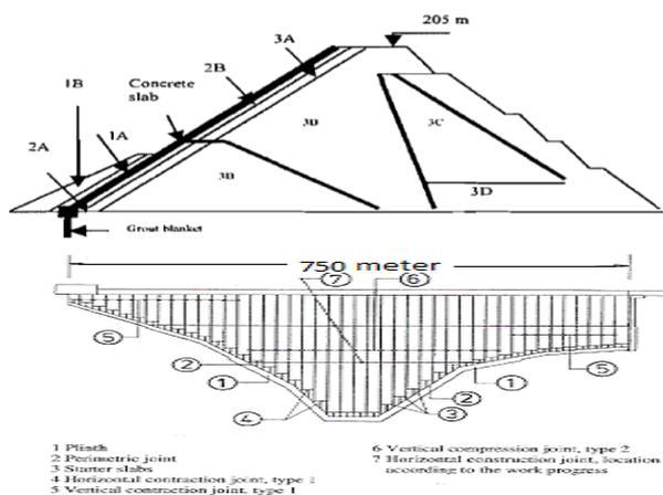
Figure 5: a) The dam section with different zones, b) Upstream face of dam,
