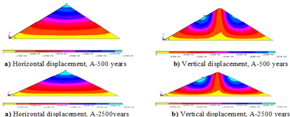
**Figure 8. Distribution of displacements in different site class for 500 years returns earthquake period**
