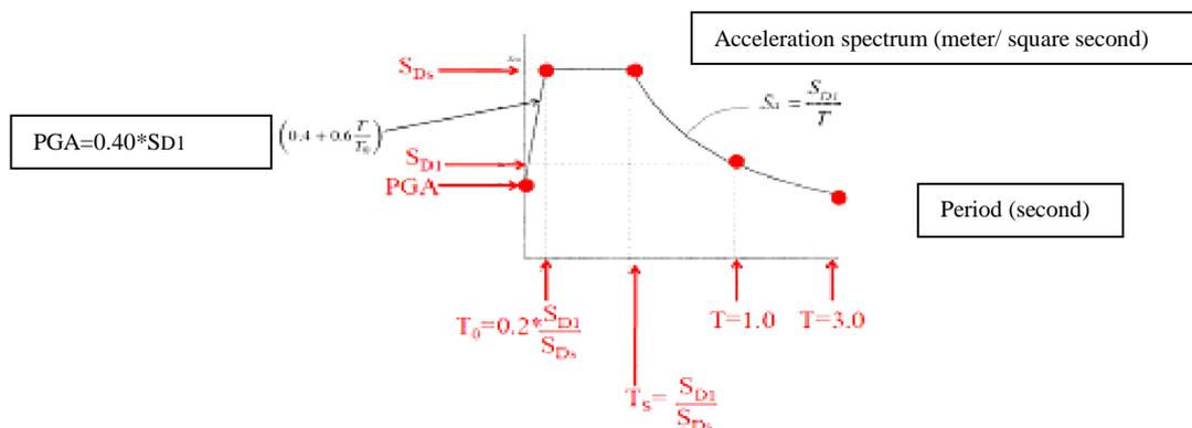
**Figure 3: ASCE Acceleration spectrum curve. The period and acceleration spectrum was matched by horizontal and vertical axis**
