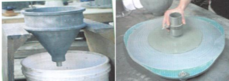
Figure 2. Flow cone and flow meter setup
