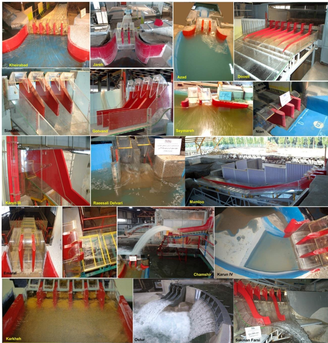
Figure 3- Images from hydraulic models of flood discharge systems in the present study
