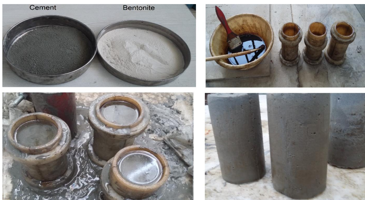
Fig. 1 - Materials and steps to prepare the sample
