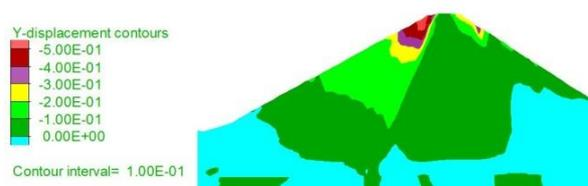
**Fig 12. Vertical displacement contours of Khoorgo earthquake**
