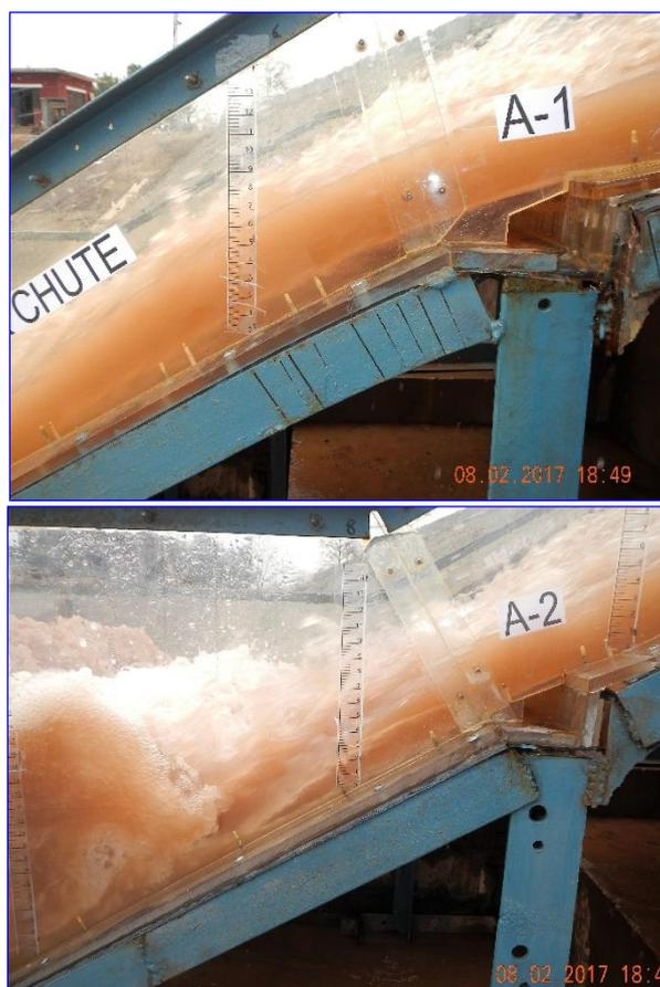
**Figure 10. Nappe profiles at aerators 1 & 2**
