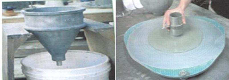
Figure 2. Flow cone and flow meter setup
