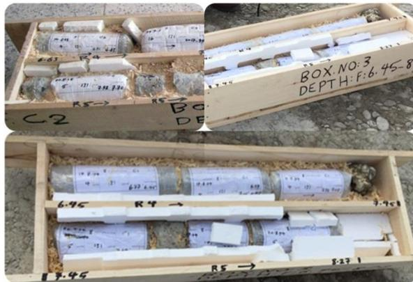
**Figure 4. Core samples of Kahir dam**
