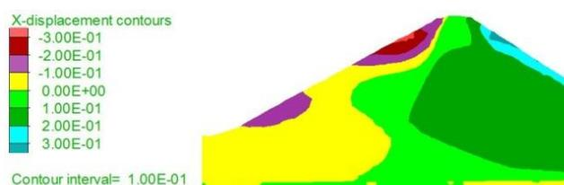
**Fig 13. Horizontal displacement contours of Khoorgo earthquake**
