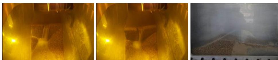
Figure 2. Centrifugal model test of clay core rockfill dam due to overtopping failure
