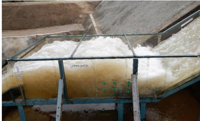
**Figure 7. View of the upper basin operation for AEP 1 in 10,000**
