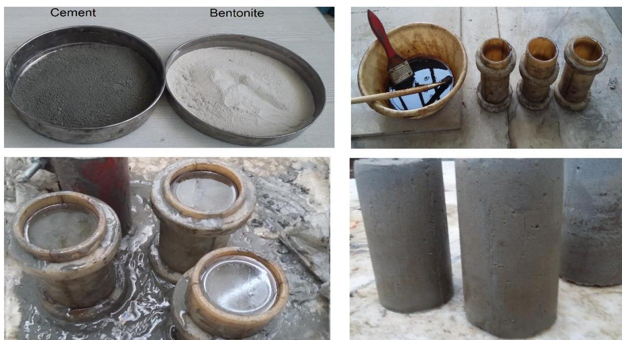
**Fig. 1 - Materials and steps to prepare the sample**
