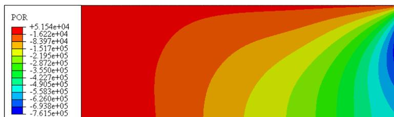
**Figure 18-Contours of hydrodynamic pressure in 13.63 second due to Kobe far field motion**
