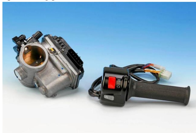
Figure 105 Ride-by-wire throttle body and throttle grip from KTM [158]
