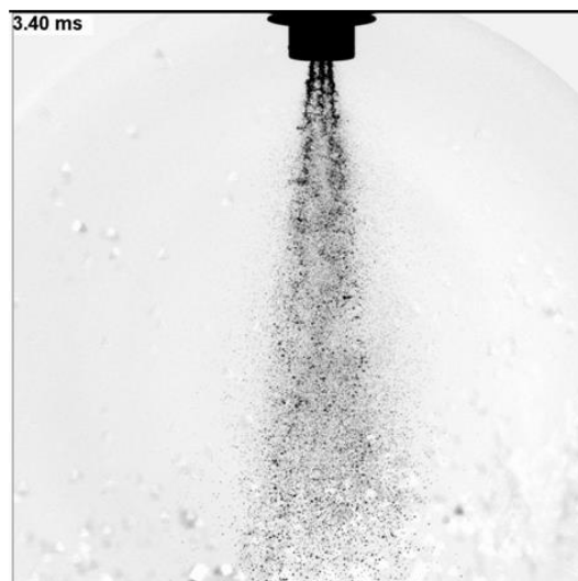
Figure 71 Fuel jet of an injector with a three-hole nozzle
