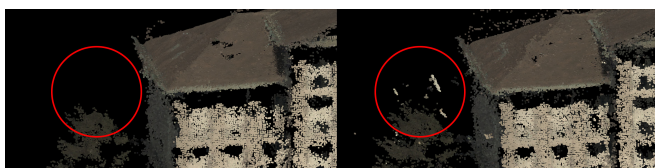
Fig. 7. Taking all TV classes into account produces point clouds containing less outliers (left), in contrast to point clouds restricted to TV classes > 1 (right).
