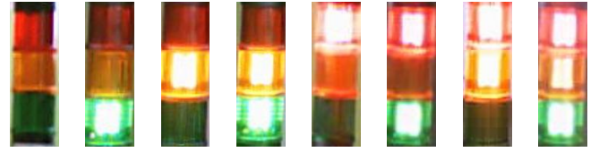
Fig. 5. Cropped traffic light by the histogram of oriented gradients detector.
