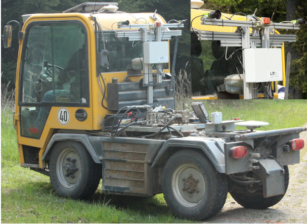
Fig. 2: Vehicle with measurement setup and DGPS-receiver
