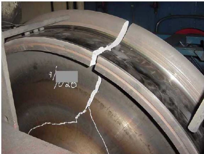
Figure 72 Thermal stress on wheel (Dr Merkel, 2005)
