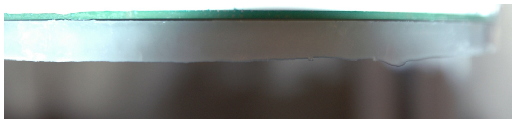
Figure 4.6: Gap between PCB (green) with a thickness of 1.6 mm and the ice layer that leads to a zero capacitance.
