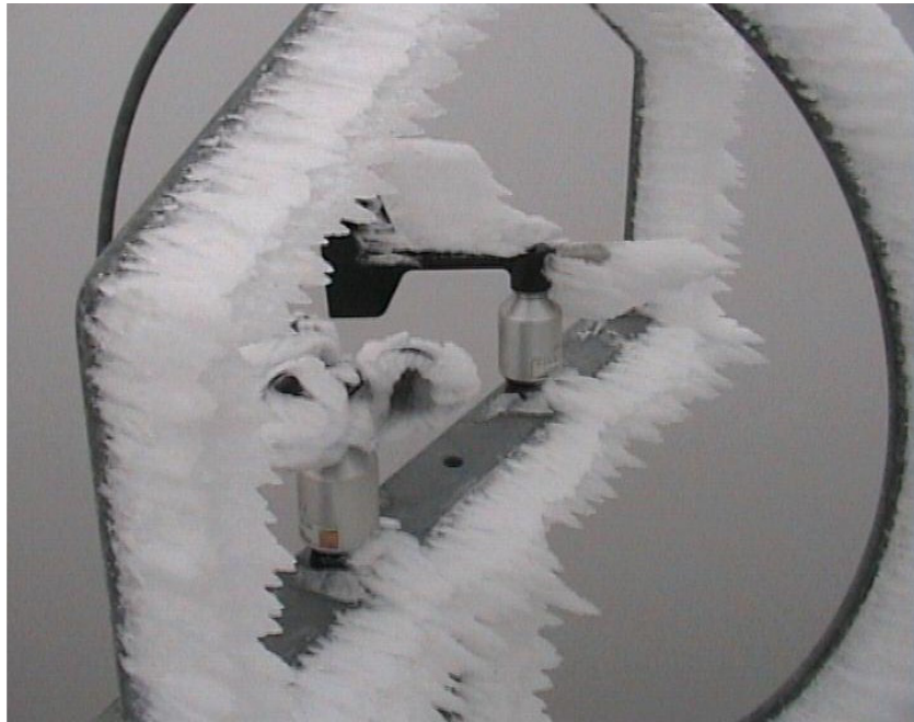
Figure 1.1: Disturbed movement of a cup anemometer and wind vane caused by ice and snow [1].
