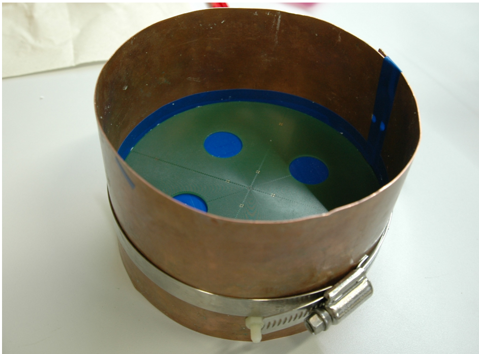
Figure 4.5: Copper sheet surrounded sensor PCB with (blue) tape covered ventilation wholes, to freeze the PCB.
