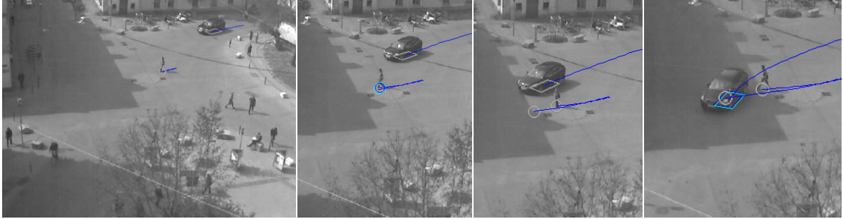
Figure 8.37: A conflict and its real- and hypothetical “no reaction” - trajectories at the shared space Sonnenfelsplatz: A Pedestrian is crossing the square at his shortest central path, priority clearly is at the car drivers side.
