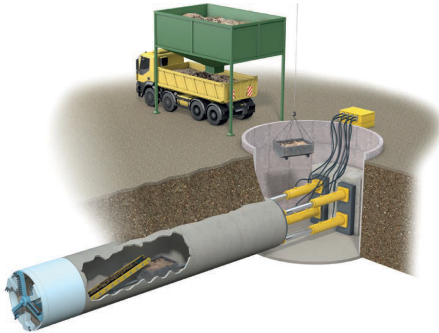
Figure 2.15: Typical pipe jacking arrangement (Pipe-Jacking-Association, 2017, p.4)
