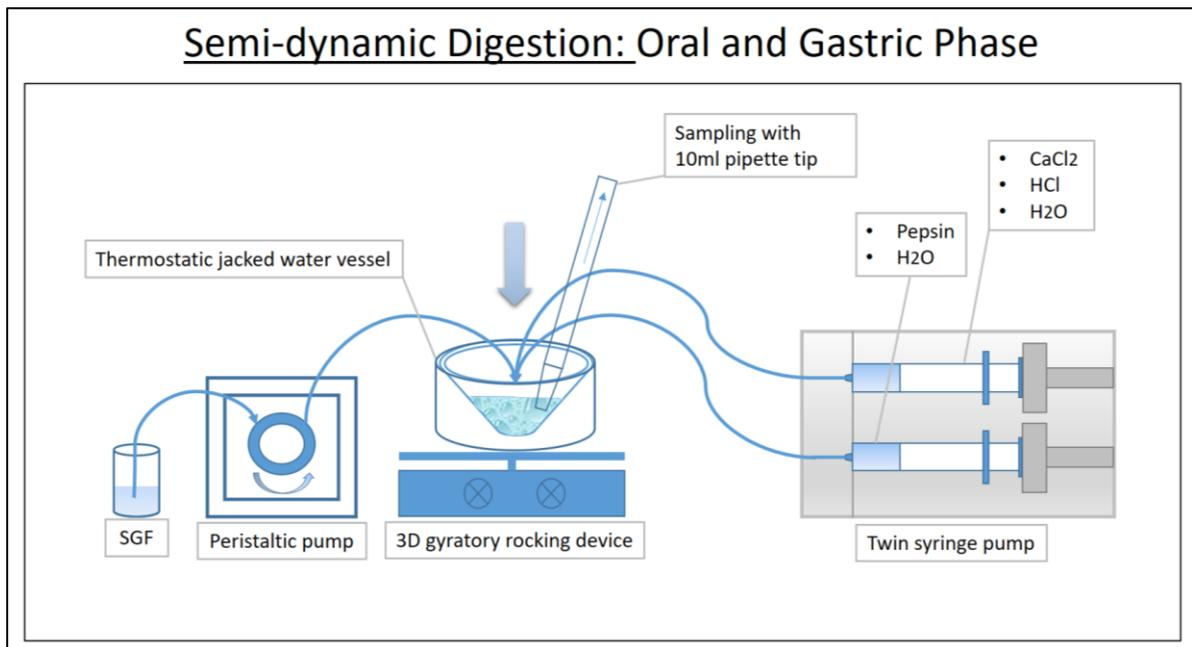
Figure 11 Schematic set-up of oral and gastric phase of semi-dynamic digestion experiments.
