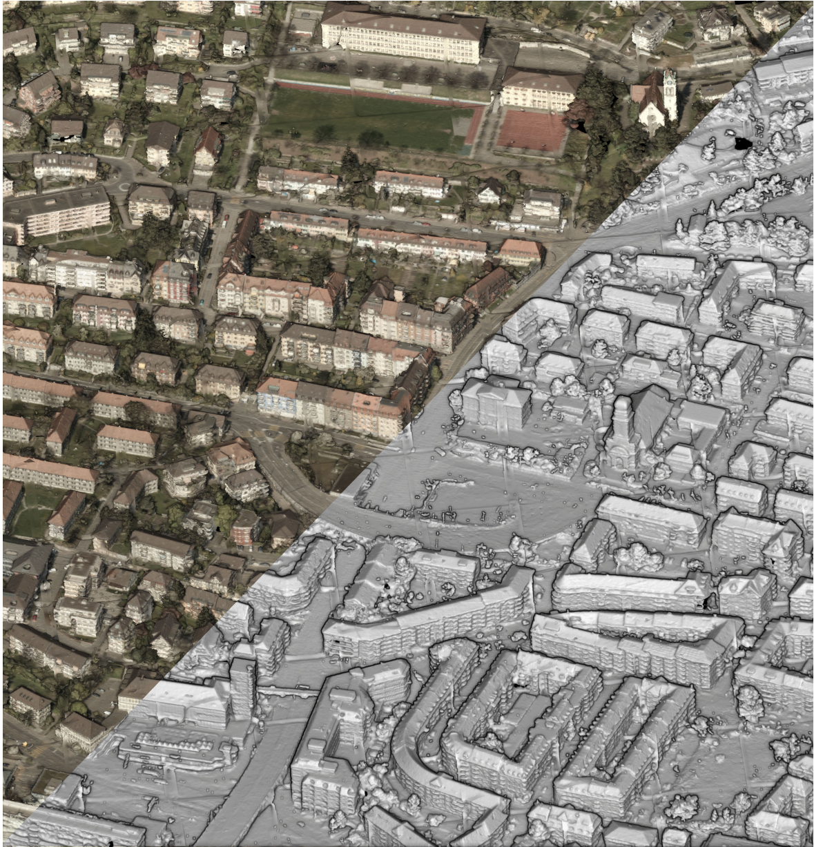
Figure 5.11: Reconstructed mesh from several fused point cloud tiles, showing the capability of the point cloud fusion method for the generation of 3D city models.
