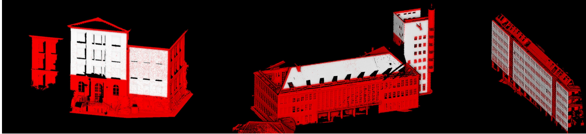
Figure 5.3: Reference TLS point clouds and extracted facade patches of two selected test areas: school building ( left ) and tower area with neighboring building ( right ).
