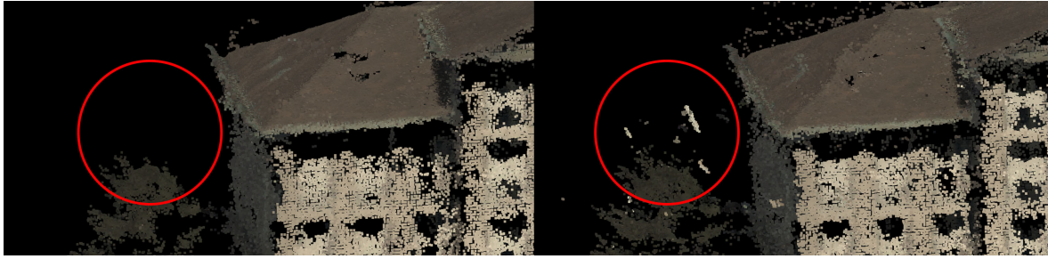
Figure 5.14: Pre-filtering of TV classes: Taking all TV classes into account produces point clouds containing less outliers ( left ), in contrast to point clouds restricted to TV classes > 1 ( right ).
