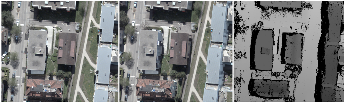
Figure 2.1: Stereo matching two epipolar rectified images resulting in a so-called disparity map ( right ) (i.e. the stereo parallaxes in epipolar direction).
