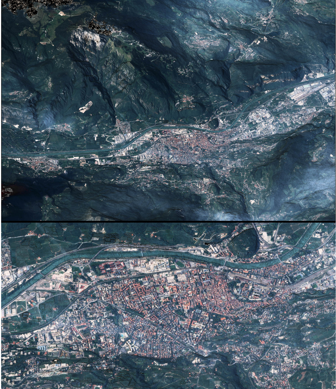
Figure 5.25: Overview of the reconstructed scene. Underlying colorized point cloud fused for visualization purpose within 4 hours by setting the approximate output GSD to 2 m.
