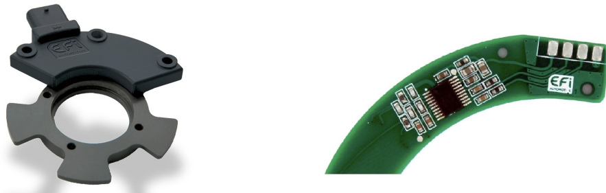
Figure 2.7.: Technical realization of an eddy current sensor (left) and evaluation electronics (right) [14].
