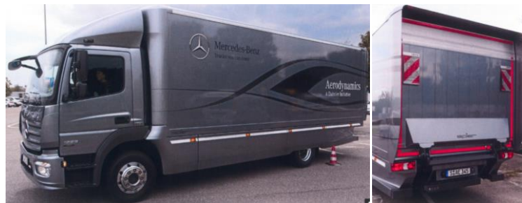
Figure 103. Delivery truck with aerodynamic improvements (174)
