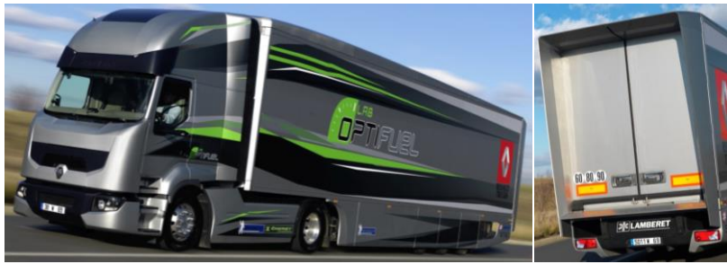
Figure 102. Tractor-trailer with aerodynamic improvements (renault-trucks.com)
