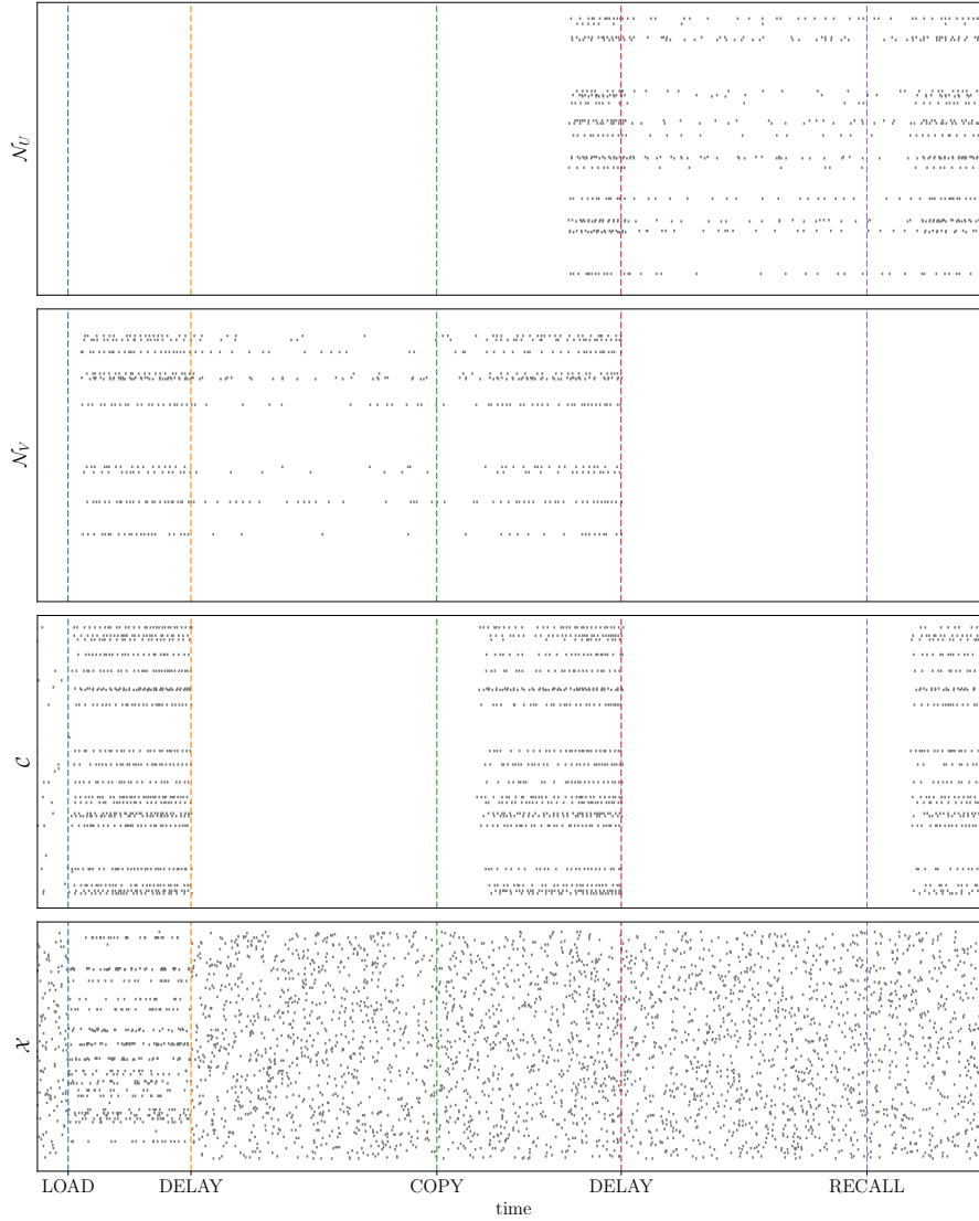
Figure 16: Spikes in input population \mathcal{X} , content space \mathcal{C} , and variable spaces \mathcal{N}_V and \mathcal{N}_U during a successfully LOAD / COPY / RECALL sequence. The beginning of each command is marked on the x-axis. The spikes of 200 neurons of each population are shown. For the three neural spaces, the neurons were randomly selected; for the input population, this is the entire population. The time axis is drawn to scale.
