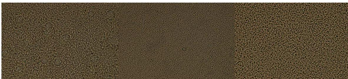
Figure S10. Optical microscopy images (50x magnification) of casted films of regenerated TMSC/LP in different ratios (left 3:1, middle: 1:1, right: 1:3)
