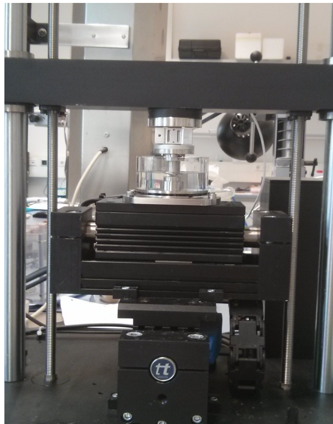
Figure 2.6: Experimental setup of the triaxial testing device. The upper part consists of the load cell which is attached to the upper specimen holder. The container is filled with PBS, which prevents dehydration of the specimen. The actuator in z-direction is located above the load cell. The other two actuators in x- and x-direction are located beneath the lower specimen holder.
