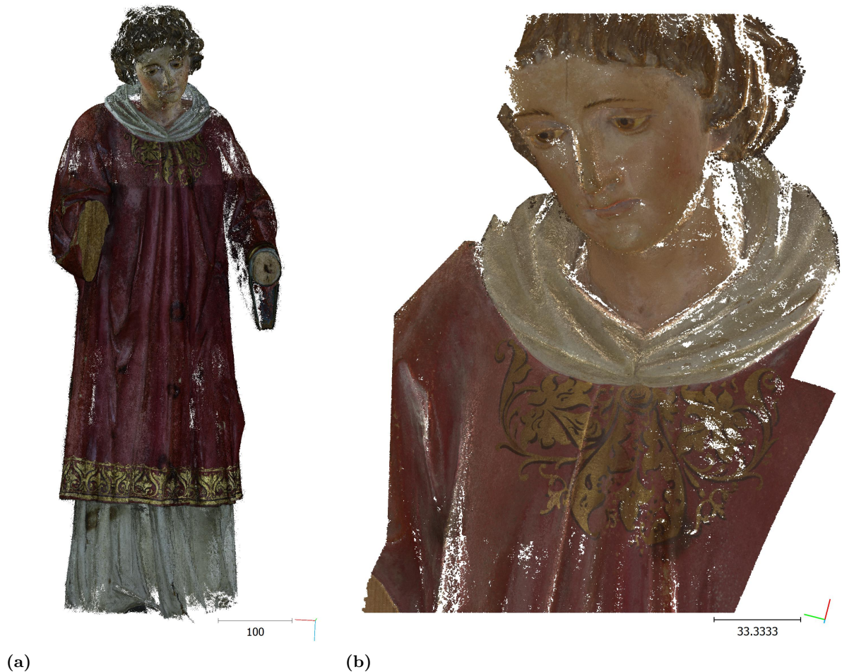
Figure 5.6: Radiometrically uncalibrated (a) and calibrated (b) 3D point clouds of a colored wooden statue (see text).
