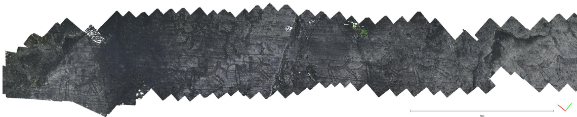
Figure 3.7: This figure shows a scan of area 10. The entire area is an elongated structure of approximately 2.6 meter length and was reconstructed using 104 images.
