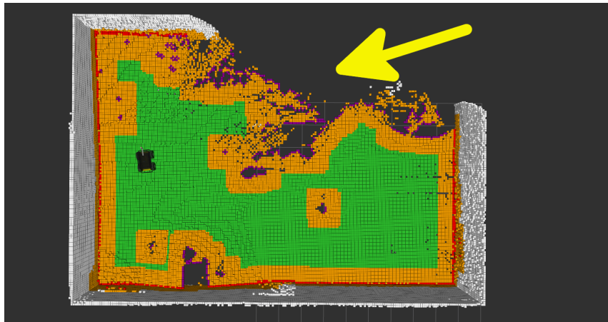
Figure 7.9: Illustration of the 3rd run of the outdoor world where some parts weren't correctly classified. The yellow arrow indicates the area that is also traversable but wasn't classified as such.
