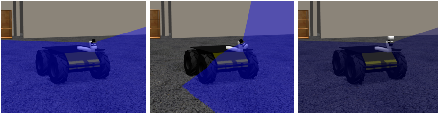
Figure 5.6: Illustration of the laser scanner alignment during one complete sweep
