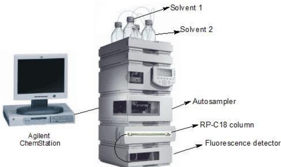
Figure 7: Setup of the HPLC system.
