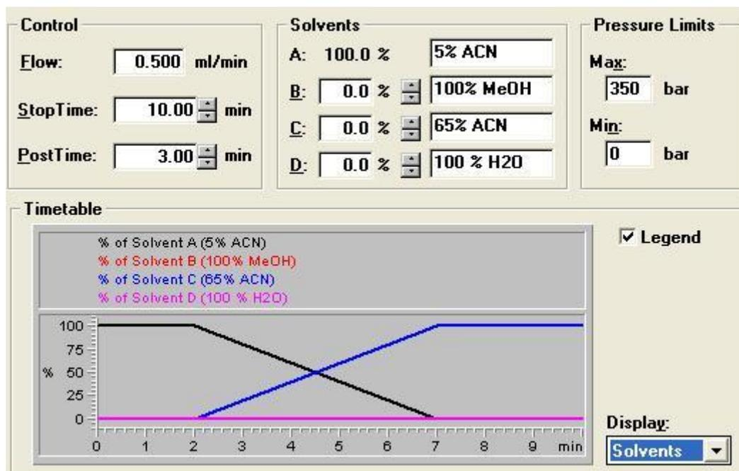
Figure 14: The gradient for method 5 was started with solvent 1 for 2 min and changes after 7 min to solvent 2. This is a screenshot from Agilent's ChemStation.
