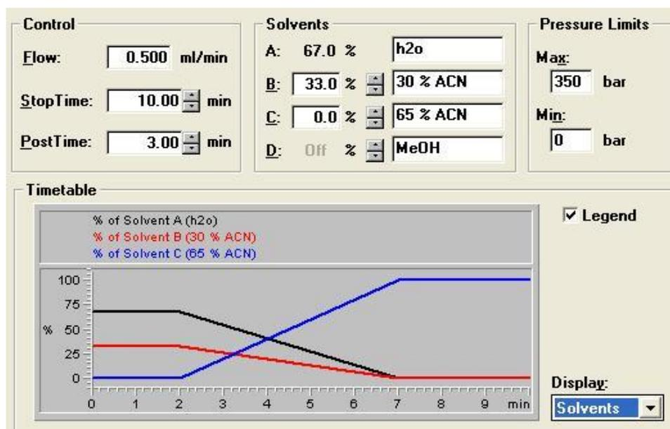
Figure 13: Gradient of method 3. 10 % ACN in solvent 1 was reached and solvent 2 stayed the same. This is a screenshot from Agilent's ChemStation.
