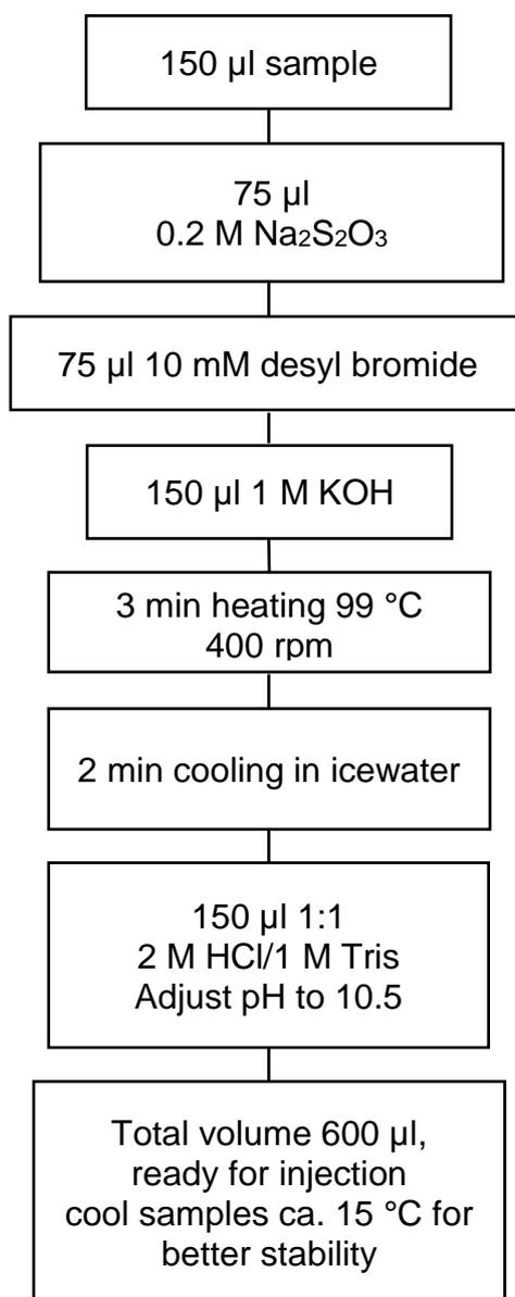
Figure 10: Flow chart for derivatization of metformin with desyl bromide.
