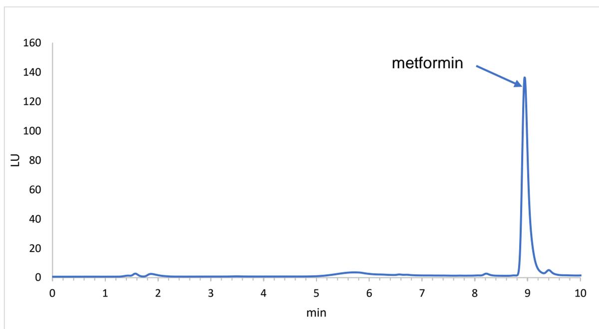
Figure 15: Method 5. 0.5 mg/ml metformin derivatized with desyl bromide in water.
