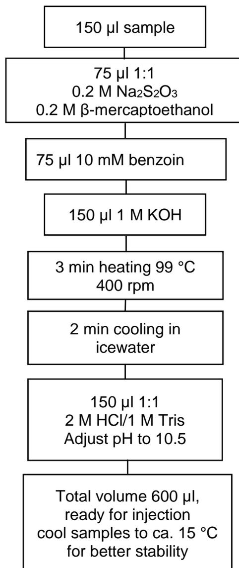
Figure 9: Flow chart for derivatization of metformin with benzoin
