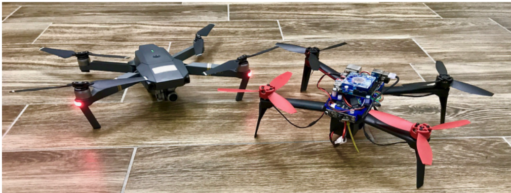
Figure 3.7: The custom built drone next to a very popular DJI Mavic Pro drone, to get a better comparison of size.
