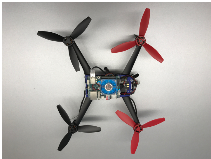
Figure 3.8: Top-view image of the assembled drone.
