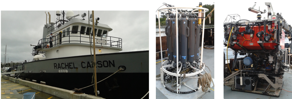
Figure 1.8: From left: Research vessel ' Rachel Carson ' operated by Monterey Bay Aquarium Research Institute (MBARI), CTD rosette with 12 water samplers and the ROV ' Ventana '.
