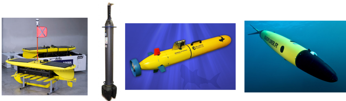
Figure 1.10: Mobile platforms from left a waveglider, a profiling float, an AUV and a glider. 86
