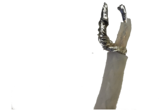
Figure 5.1: Example of a self constructed measurement connection
