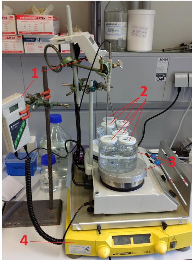
Figure 3.9: Picture of the custom build setup for the dissolution testing. Six specimen jars (2) were placed into temperature controlled (1) water baths, standing on heating plates (3), which were mounted on a moving table (4) to facilitate mixing of the dissolution medium.
