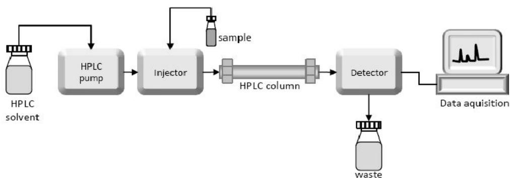
Figure 3.10: Schematic diagram of the HPLC instrumentation. Reprinted from [12].
