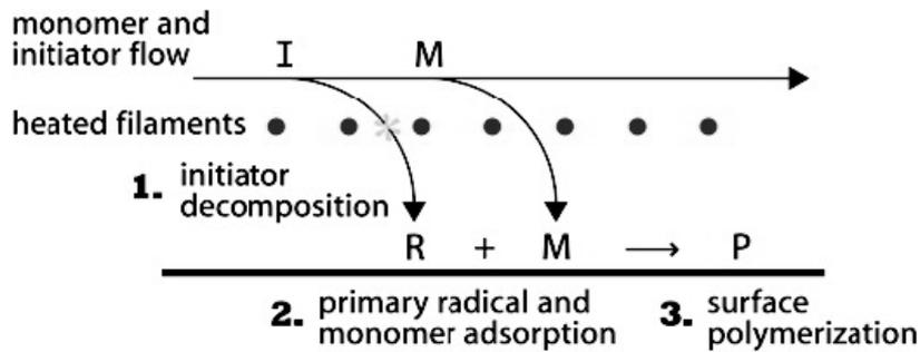
Figure 2.6: Illustration of the three major steps for the iCVD process. Adapted from [16].
