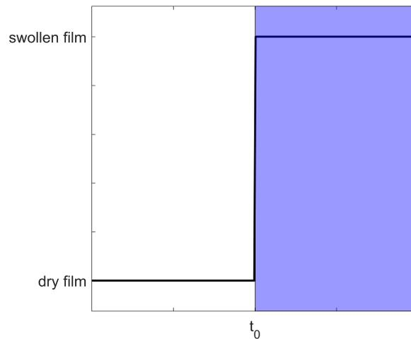
Figure 3.7: Schematic drawing of a swelling experiment of a hydrogel thin film. At  $t_0$  the liquid is applied to the liquid cell where the thickness of the film increases from the dry to the swollen state.
