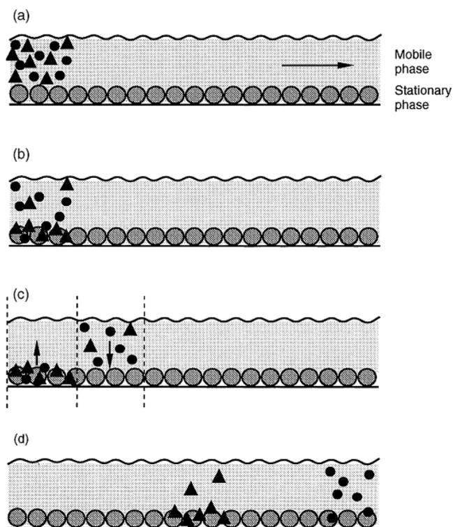
Figure 2.7: Graphical representation of the separation process in the chromatographic column of a HPLC apparatus. Reprinted from [18].
