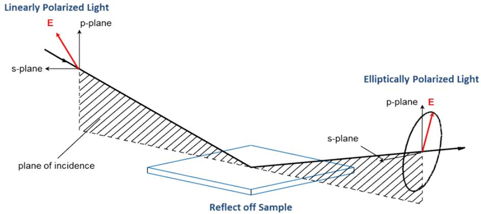
Figure 3.4: Schematic drawing of the light path occurring during an ellipsometry measurement. Reprinted from [15].
