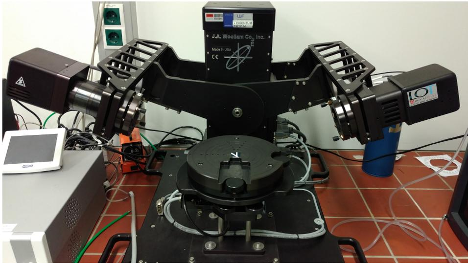
Figure 3.5: The ellipsometry setup with the basic stage attached for measurements in air.
