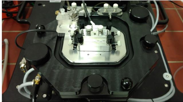
Figure 3.6: Close up picture of the liquid cell that can be attached on to the stage of the ellipsometer for in-situ thickness measurements of the hydrogel layer in liquid environment.
