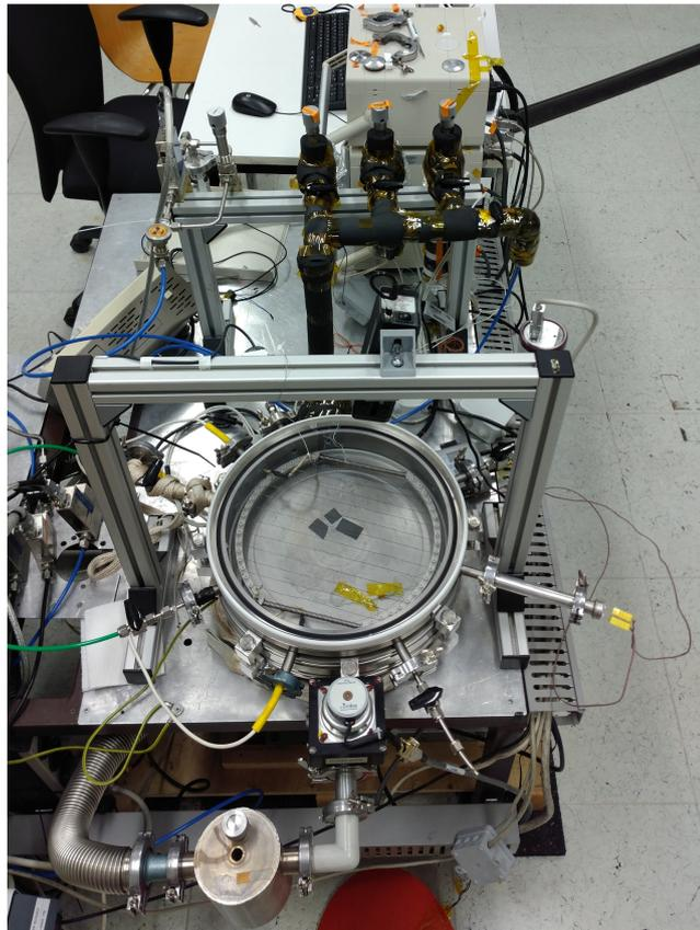
Figure 3.2: Picture of the custom build iCVD reactor standing in the 3<sup>rd</sup> floor lab at the institute of solid state physics at the TU Graz.
