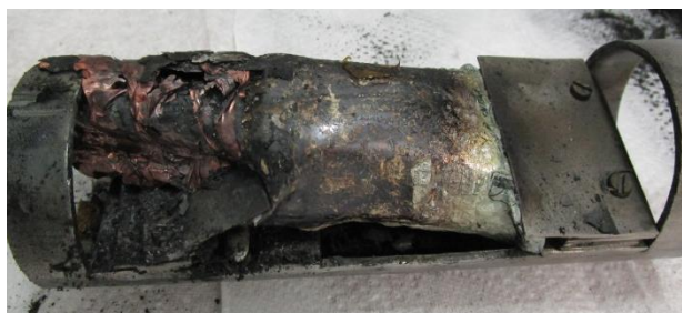
Figure 32: destroyed LG cell
