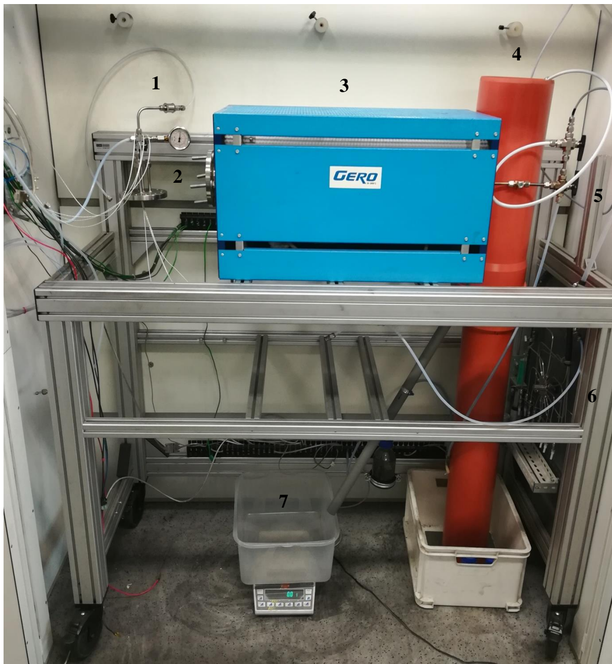
Figure 6: Complete test rig under the fume hood, 1) inert gas inlet and manometer, 2) flange, 3) tube furnace, 4) water displacement apparatus, 5) gas exhaust valve, 6) 16 port gas sampling valve, 7) scale.
