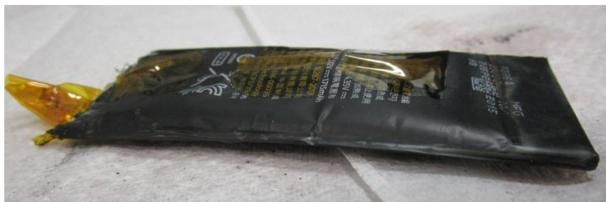
Figure 37: expanded iPhone cell after experiment with the DC heating device and 70 W oven performance
