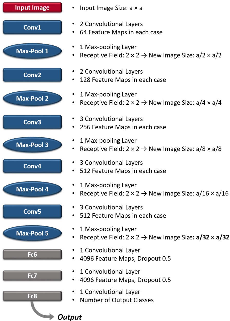
Figure 53: Network architecture of the TF-Slim VGG-16 model.
