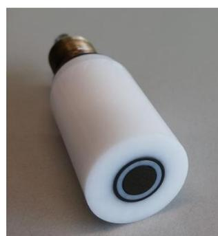
Figure 25: Rotating ring-disc electrode with Pt ring and glassy carbon disc.
