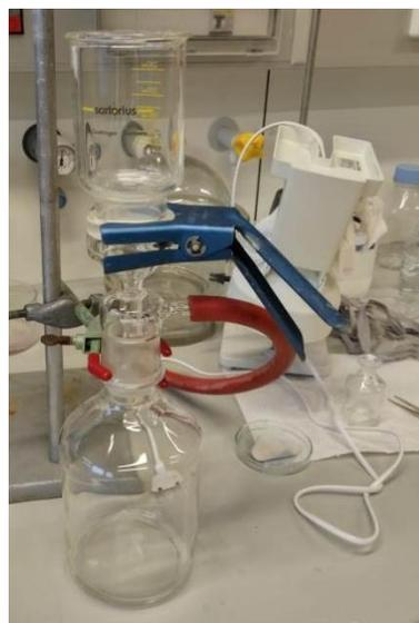
Figure 23: Arrangement of the filtration equipment.
