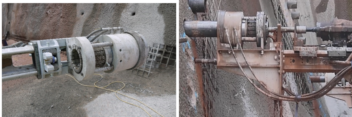
Figure 5 AT – Squeezing Unit with remote-controlled hydraulic wrench.
