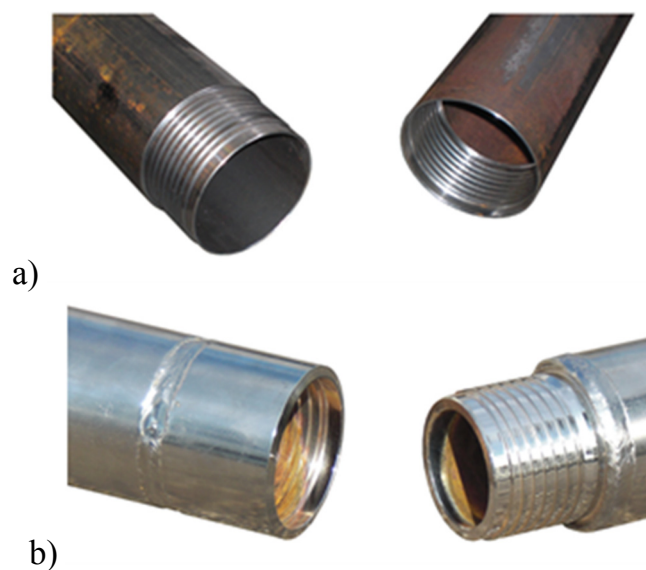
FIG 4 a) standard threaded connection and b) threaded nipple connection.
