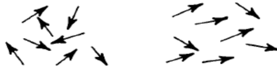
Figure 8: Orientation polarization, which displays the orientation of permanent dipoles. Left: unpoled state and right poled state. [1]
