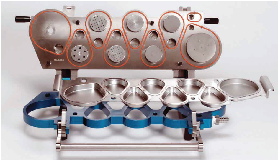
Fig. 7: Open NGI with the cup trays and the injector nozzles on the cover [66]
