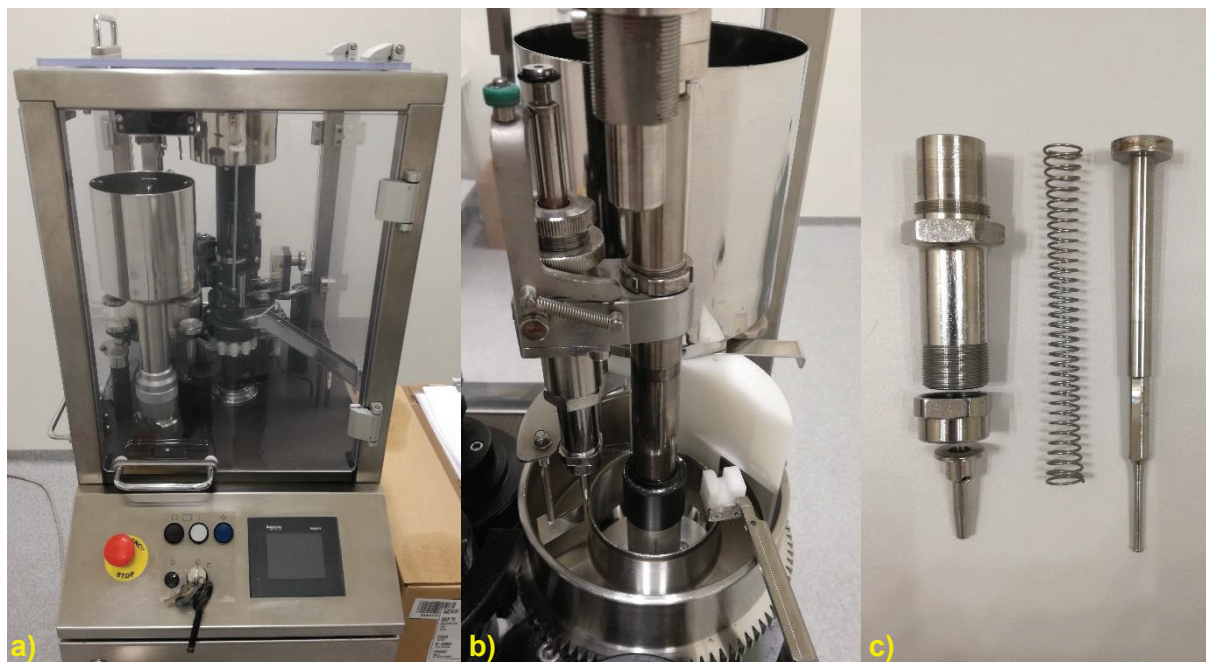
Fig. 5: a) Labby capsule filling machine b) Assembled capsule filling unit (with dosator, rotating container and scrapers) c) dosator parts in detail
