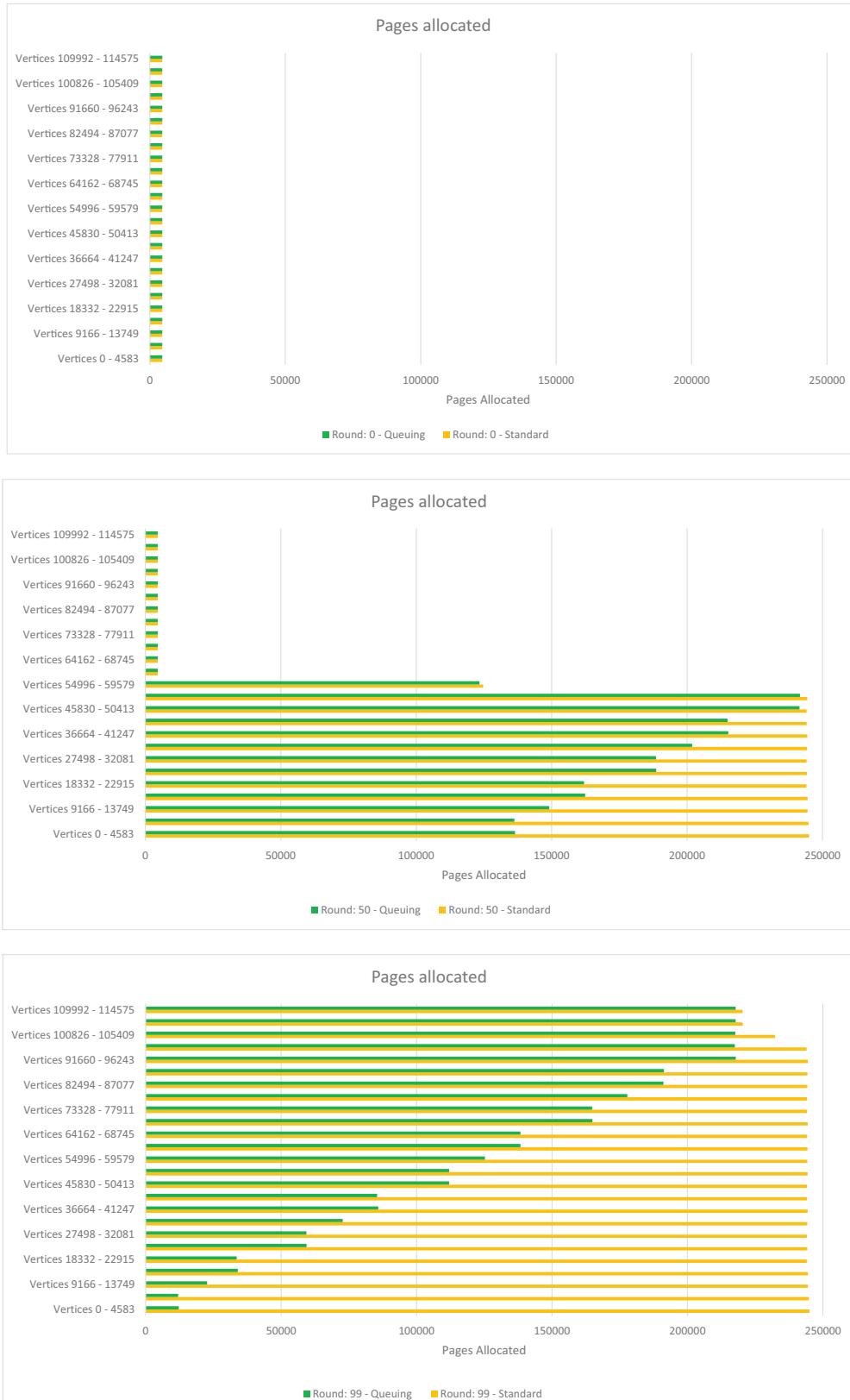
Figure 4.2: Page allocation count over 100 update iterations with sweep update strategy. The queuing approach can return empty pages once the insertions target different sections.
