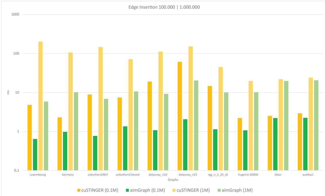
Figure 6.1: Performance measurement for edge insertions, using a batch size of 100.000 and 1.000.000, showing cuSTINGER compared to the best aimGraph implementation
