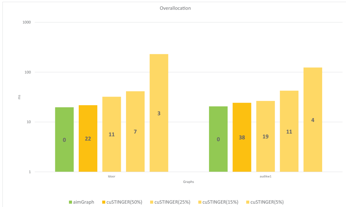
Figure 6.2: Vertex Insertion with batchsize 1.000.000, cuSTINGER is depicted with different overallocation factors (50%, 25%, 15% and 5%), the numbers in the bars represents the average number of additional elements allocated per adjacency with this factor
