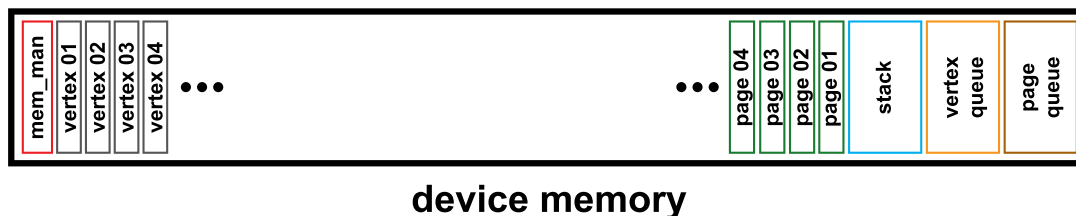
Figure 3.1: Visualization of the device memory layout as managed by the memory manager
