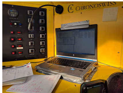
Figure 4.6.: Mounted computer to record data (selfmade).
